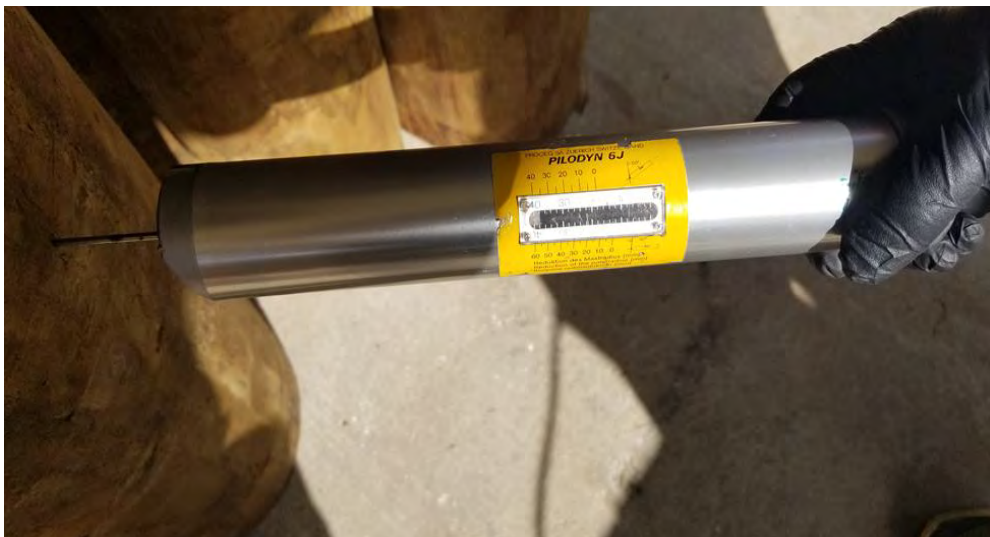
Figure 1. Pilodyn Testing of Treated Poles
